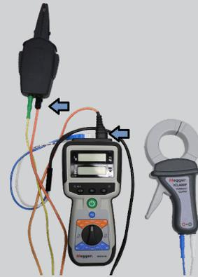
Connect the Capacitive Pick Up ground to earth.
