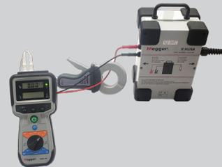
Connect the Capacitive Pick Up to the positive lead of the transmitter after the AC Filter box.
