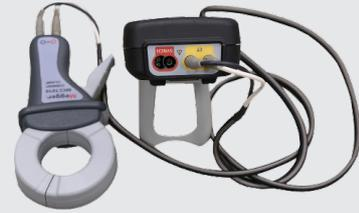
Connect the sync cable between the receiver and the Capacitive Pick Up.
