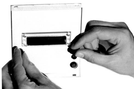
Fig 38: Unscrewing the printer front cover
