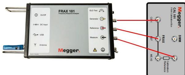
When looking at standard view Magnitude Curve should be around -80 dB between 10 Hz – 100 kHz.
