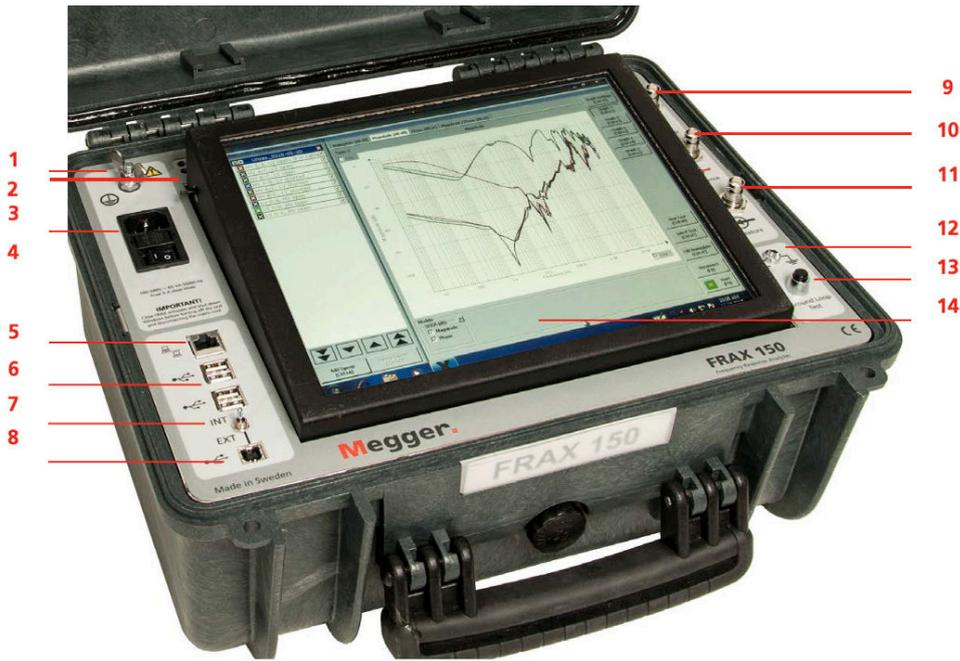
1. **⚡ Ground (Protective earth) connector** Always connect the instrument to station earth/ ground using the separate earth/ground cable. The separate earth/ground wire should be the first connection made and the last removed.
