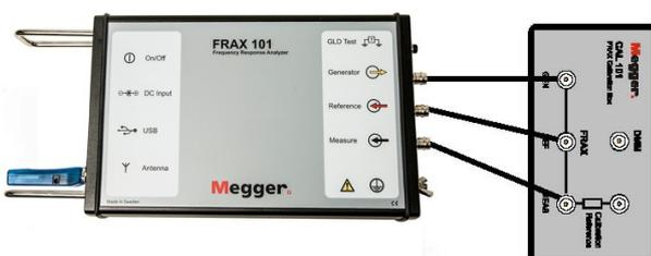
Measure from 10 Hz to 10 MHz and the measured data should be 0 dB with a maximum deviation of +/-0.1 dB.
