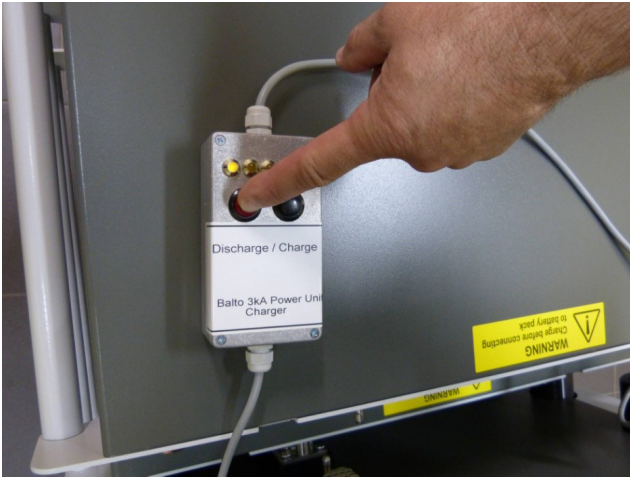
Fig 39: Discharging a DC Current Generator.
