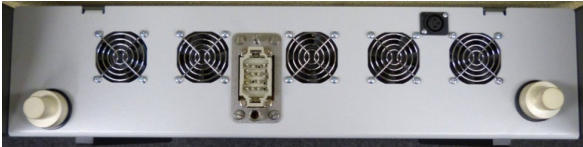
Fig 54: DC Current Generator vents
