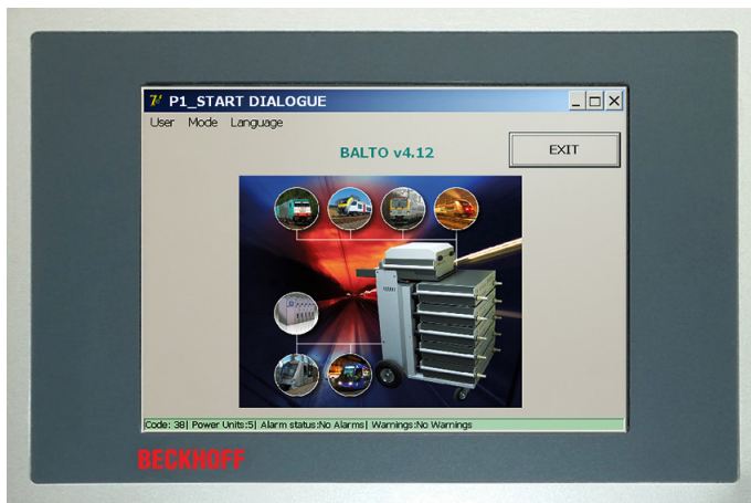
Fig 19: Control Panel: Touch Screen Display - HMI
