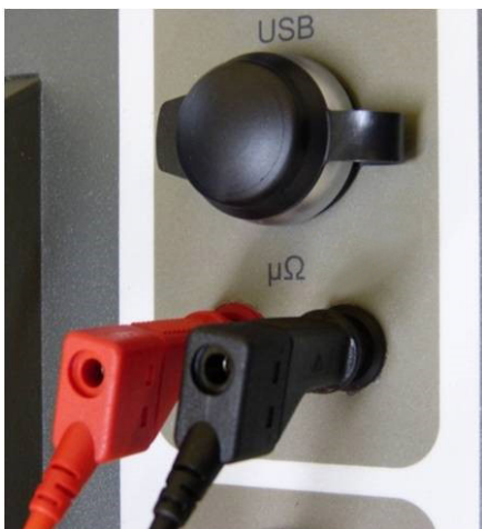
Fig 36: Control Panel: \mu\text{Ohm} measurement connection.
