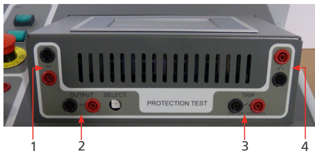
Fig 8: Control Unit: Interface DC Protection Relay.
