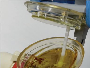
Fig 6: Baffle plate must come in contact with the oil
