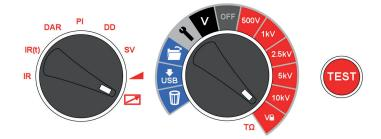
Instrument controls are simple to operate. The central rotary switch incorporates the OFF position. The left hand rotary switch selects insulation test type. The TEST button starts and stops a test. Image depicts instrument setup for Remote Control mode.
