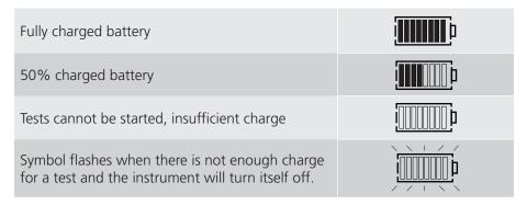
When mains power is present the indicator shows the battery is being charged by animating the segments of the bar graph.
