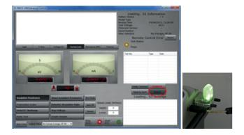
To activate the Import/Live Stream Control application click the Import soft button (circled) in the remote control application
