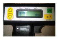
When the data transmission is complete, the following screen is displayed. This screen will allow you to select the data path you wish to save the transmitted data to.
