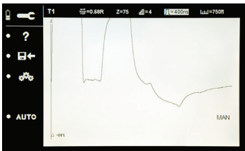
Figure 5 - Pulse Width and Dead Zone
