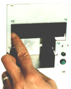
Fig 40: Removing the ribbon cartridge
