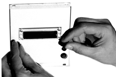
Fig 38: Unscrewing the printer front cover
