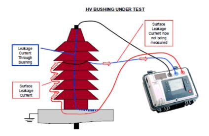
Measured current = insulation leakage current only. Surface leakage current is "guarded out".
