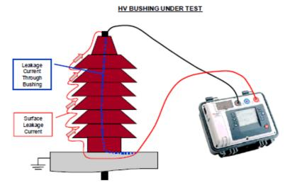
Measured current = surface leakage current + insulation leakage current
