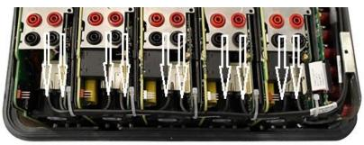
Figure 310 Communication Cable Connections 5 Channel Unit
