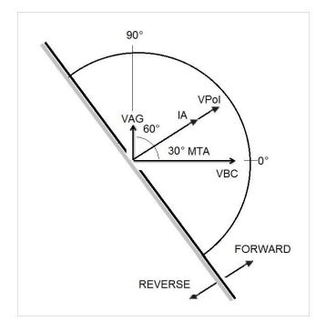
As figure shows for overcurrent directional will operate, when angle current reach the polarizing voltage, this polarizing voltage comes from VA-B reference voltage angle previously configured by user, plus MTA configured in the relay and RTMS software.
