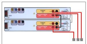
Figure 223 Three Phase Open Delta Connections
