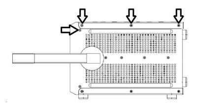
Figure 285 Top Cover Removal, Side Screws
