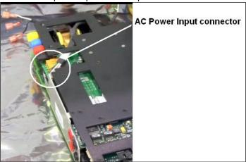
Look for possible discoloring of the wires and connector indicating overheating. Make a general observation of the VIGEN module looking for any obvious damage caused by a short circuit or other possible signs of trouble.
