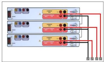
Figure 224 Three Phase Four Wire Voltage Test Connections
