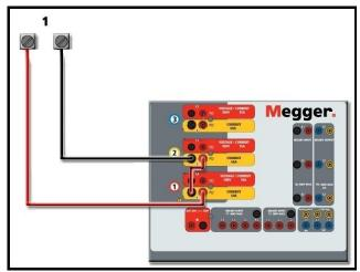
Figure 279 Series Two Currents with Floating Output Unit
