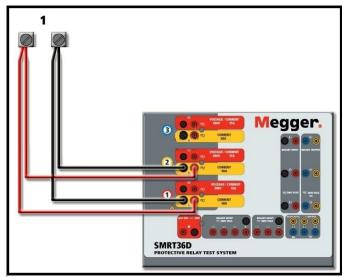
Figure 36 Two Currents in Parallel (on SMRT36D)
