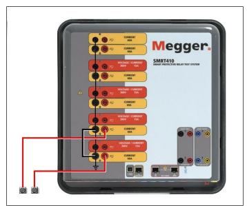
Figure 301 Series of Two Current Channels with Grounded Common Returns
