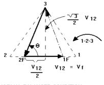
NORMAL BALANCED CONDITION V 12 = V 31 = V 23
