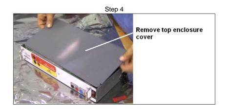
CAUTION: From this point on observe proper ESD procedures. Be careful when moving the VIGEN module as it is a tight fit, and it is possible to damage components upon extraction from or installation to the bottom half of the enclosure.
