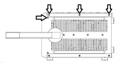
Figure 263 Top Cover Removal, Side Screws
