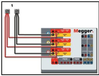
Figure 276 Parallel of All Three Current Outputs
