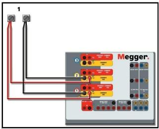
Figure 278 Two Currents in Parallel
