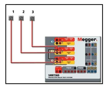
Figure 261 Three Phase Open Delta Connections
