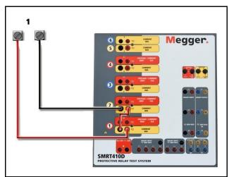
Figure 322 Series Two Currents with Floating Output Unit
