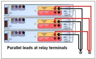
Figure 218 Parallel of Three SMRT1 Current Outputs
