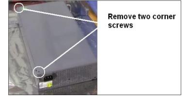
Step 1 Disconnect the power cord from the unit, and remove top corner screws.
