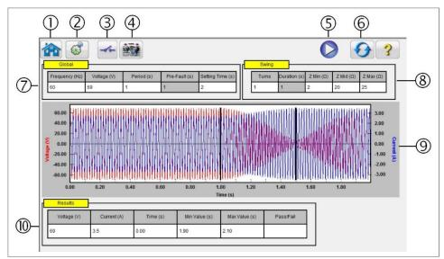
Figure 162 Example COMTRADE Playback Test Screen
