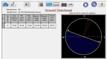
Figure 87 Example Ground Directional Test Screen
