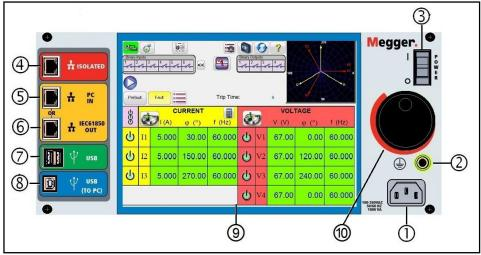
Figure 270 SMRT46D Front Panel
