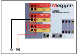
Figure 235 Series Two Currents with Floating Output Unit
