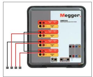
Figure 305 Three Phase Four Wire Test Connections
