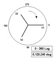
Figure 32 Negative Sequence Phase Rotation Diagrams
