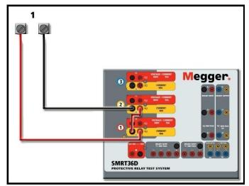
Figure 37 Series Two Currents with SMRT36D Floating Outputs
