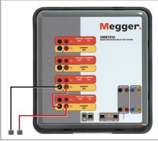
Figure 300 Series Two Currents with Floating Output Unit
