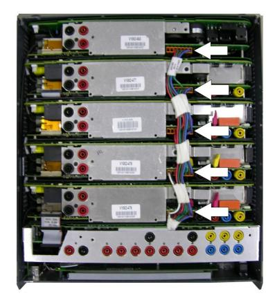
Figure 330 Amplifier Power Connectors for 5 Channel Unit
