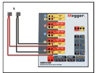
Figure 321 Two Currents in Parallel
