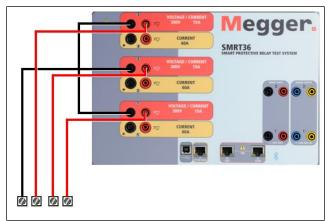
Figure 240 Three Phase Four Wire Test Connections
