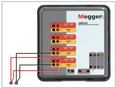
Figure 299 Two Currents in Parallel
