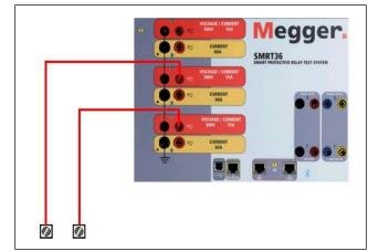
Figure 238 Series of Voltage Channels with Grounded Common Returns
