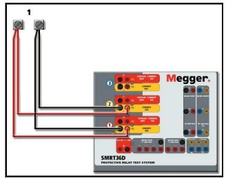
Figure 256 Two Currents in Parallel
