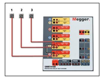
Figure 326 Three Phase Open Delta Connections
