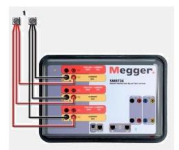
Figure 232 Parallel of All Three Current Outputs
