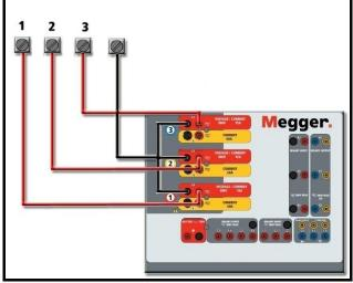
Figure 284 Three Phase Four Wire Test Connections
