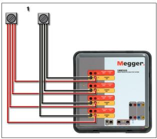
Figure 297 Parallel of Four Current Outputs
