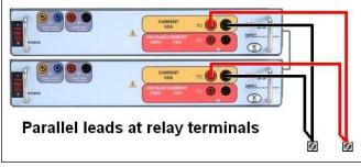
Figure 220 Two Currents in Parallel
