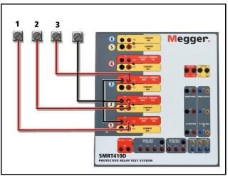
Figure 327 Three Phase Four Wire Test Connections
