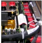
Figure 246 VIGEN1 to Front Panel Cable
