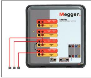
Figure 304 Three Phase Open Delta Connections
