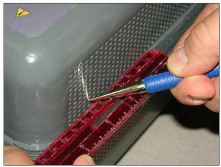
Figure 308 Leveraging the cover from the enclosure
