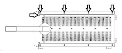
C. Remove the four screws located on the top back side, then up to six screws located on the top cover, see the following figure.
