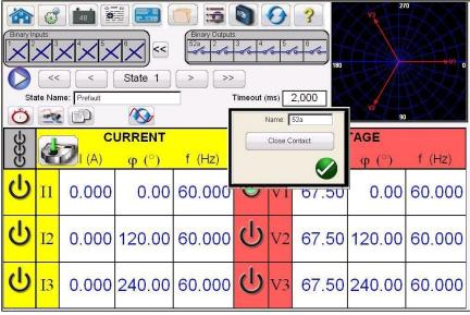
Figure 96 Binary Output Setting Screen
