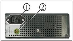
Figure 212 SMRT1 Power Input Panel
