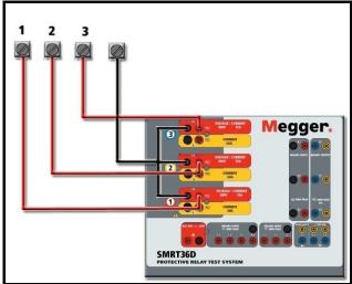
Figure 262 Three Phase Four Wire Test Connections
