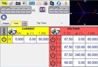
Figure 277 Manual Test Screen – Single Phase Operation
