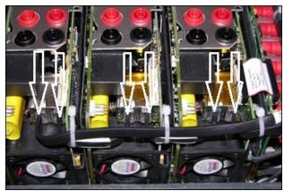
Figure 245 Communication Cable Connections
