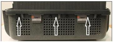
Figure 306 SMRT410 Top Cover Securing Screws11
