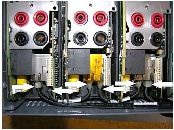
Figure 267 Communication Cable Connections
