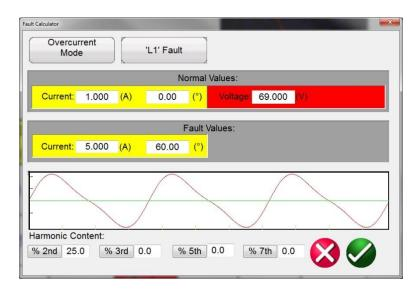
Figure 23 Fault Calculator Harmonic Current Waveform
