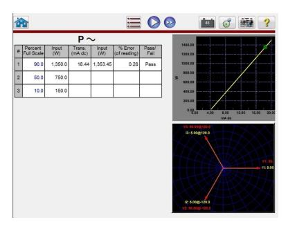
The transducer output section displays the equivalent output in the select type value (Reading V, A, Watts, VA, etc.). Depending on the desired measurement set in the setting screen the % Error will be either of range, or of reading. From this the Pass/Fail will be determined and displayed.
