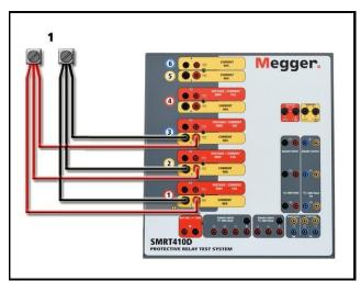
Figure 319 Parallel of Three Current Outputs
