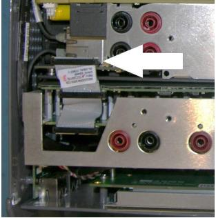
Figure 332 VIGEN1 to Front Panel Cable
