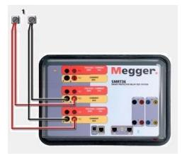
Figure 234 Two Currents in Parallel
