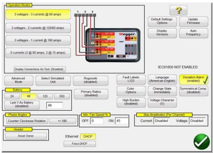
Figure 7 STVI Example Configuration Screen for SMRT36 Note: the picture will change depending on type of unit detected
