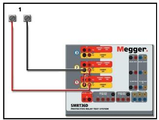
Figure 257 Series Two Currents with Floating Output Unit
