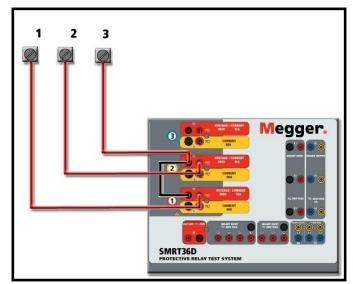
Figure 41 SMRT36D Three Phase Open Delta Connections
