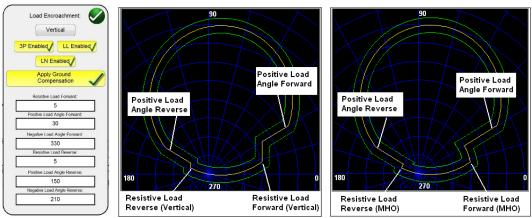
Figure 103 Load Encroachment Settings and Examples
