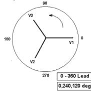
Figure 31 Positive Phase Rotation Diagrams
