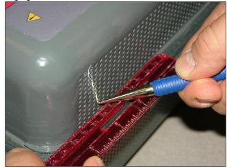
Figure 243 Leveraging the cover from the enclosure
