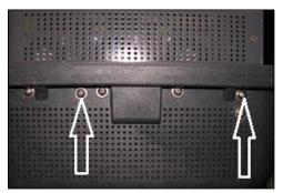
Figure 241 SMRT33/36/46 Top Cover Securing Screws®
