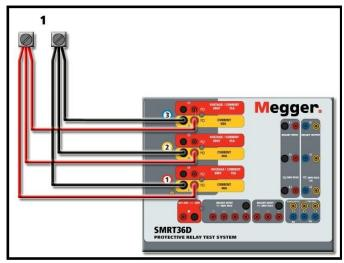
Figure 34 Parallel of Three Current Outputs (SMRT36D)
