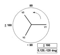
Figure 33 Positive Phase Sequence Rotation Using ± 180°
