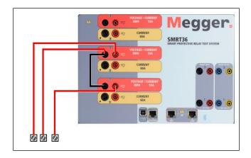
Figure 239 Three Phase Open Delta Connections
