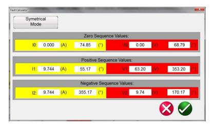
Figure 26 Symmetrical Input Setting Screen
