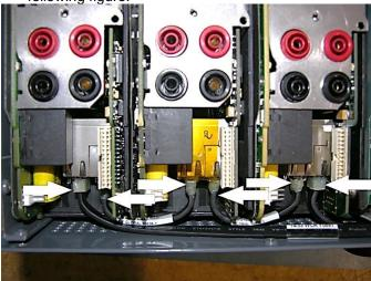
Figure 289 Communication Cable Connections
