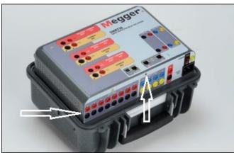
Figure 242 Top Panel Removal Front Panel Screws
