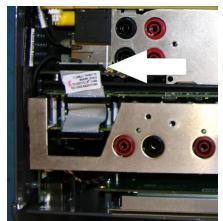
Figure 290 VIGEN1 to Front Panel Cable
