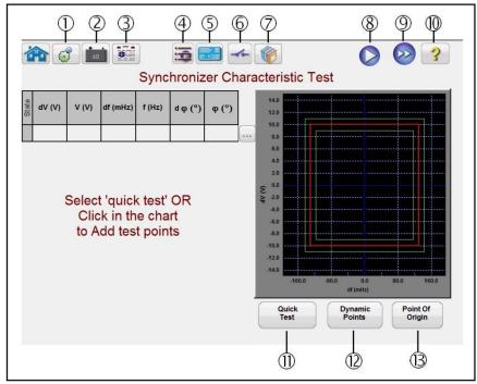
Figure 127 Synchronizer Characteristic Test Selection Screen
