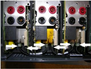
Figure 331 Communication Cable Connections
