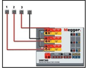
Figure 43 SMRT36D with Floating Returns, Three Phase Four Wire Test Connections
