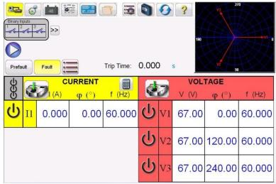
Figure 35 Manual Test Screen – Single Phase Operation
