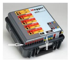
Figure 307 Top Panel Removal Front Panel Screws
