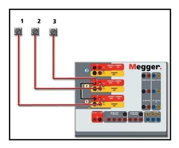
Figure 283 Three Phase Open Delta Connections
