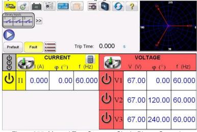
Figure 255 Manual Test Screen – Single Phase Operation
