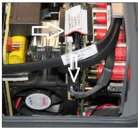
Figure 311 VIGEN1 to Front Panel Cable
