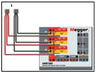
Figure 254 Parallel of All Three Current Outputs
