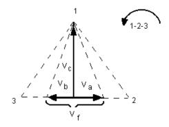
Balanced or Unbalanced Fault T-Connection
