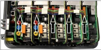
Figure 309 VIGEN Power Connectors for 5 Channel Unit
