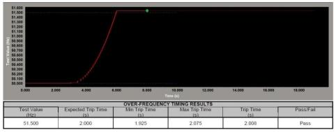
Figure 140 Over Frequency Timing Test
