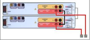
Figure 222 Series of Voltage Channels
