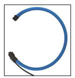
3. Place the flexible coil around the cable or buss bar to be measured and close the coil by clipping together the contacts.
